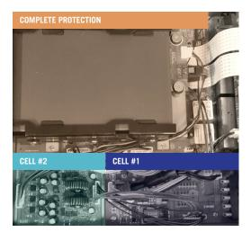
In addition, the isolated power block design protects the main hard drive from vehicle power supply issues, such as an overvoltage event or loss of power. If external power is lost, the internal power supply will ensure all data is written to the disk before shutting down, minimising lost video footage.
